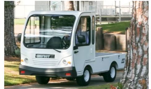
Taylor-Dunn is proud to announce an addition to its line of ergonomic BIGFOOT electric vehicles. The new BIGFOOT XL is a utility vehicle with a larger operator's compartment, hill climbing gusto, speed up to 18 mph, and all-wheel hydraulic disc brakes.
