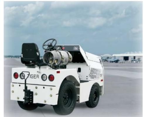
Our Tiger Cub tow tractor is designed to provide a compact and highly maneuverable solution for your towing requirements demanding 3,000-5,000 pounds (13-23 kN) of drawbar pull.
