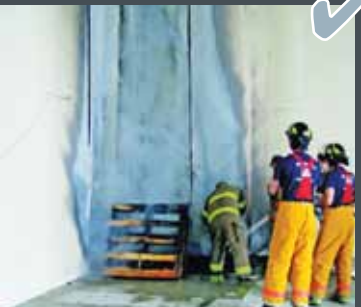
Result: Pass 25 ft. High Corner Test
