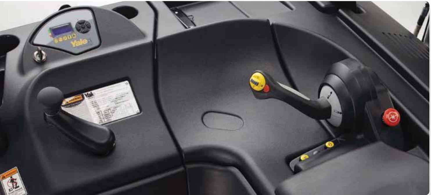
**Yale® iSi Technology™** - Offers familiar, consistent interface among other Yale® warehouse trucks, enabling easier operation and service. Ties together functionality, software, diagnostic codes and similar interfaces, and is Yale Vision compatible.
