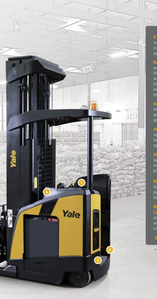
**E-Z RIDE FLOOR** – Durable rubber isolator floor system provides a comfortable ride to help keep operators focused and productive
