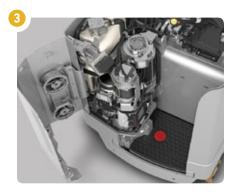
ACCESS DOOR AND COVERS provide technicians tool-free access to motors and controls.
